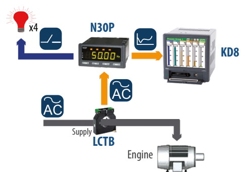
MEASUREMENT, ALARMING AND LOGGING OF LOAD CURRENT FOR A 1-PHASE ENGINE
